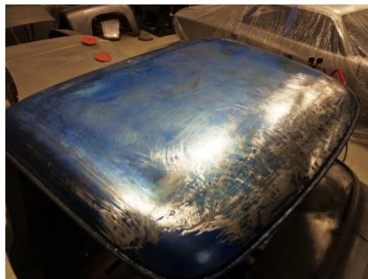
Before and after shrinking disc applied to the roof of a 1956 F100
