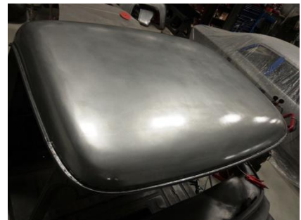
Before and after shrinking disc applied to the roof of a 1956 F100
